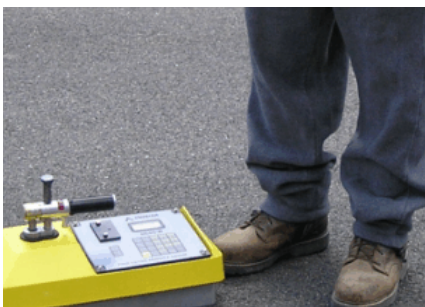
Nuclear Density Gauge to test the finished pavement to ensure proper compaction.
